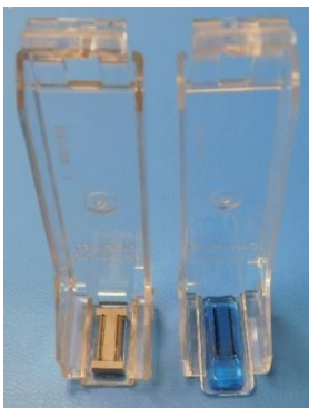
Figure 3 - Clips for aqueous (left) and solvent (right) cartridges
