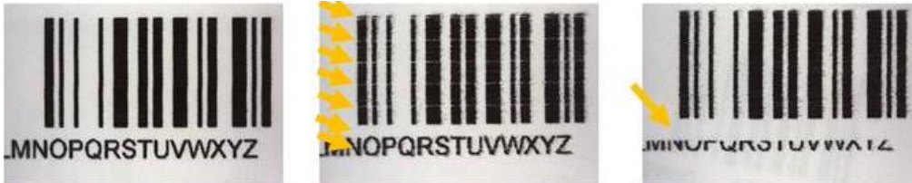
Figure 8 - Barcode segment examples: no unintended white lines (left), equally spaced unintended white lines (multiple arrows, middle), and single block of unintended white lines (single arrow, right)
