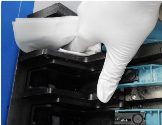
Figure 12 - Example of dabbing the pen pocket with a lint free wipe
